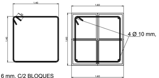
**DETALLE DE ARMADURA DE COLUMNAS DE B, DE HORMIGÓN**
