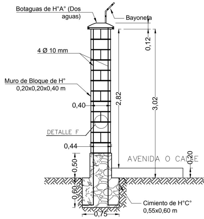
**CORTE COLUMNA DE BLOQUES DE HORMIGÓN**
